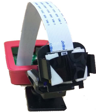
Fig.7: The image processing unit used for the motion tracking of the target
